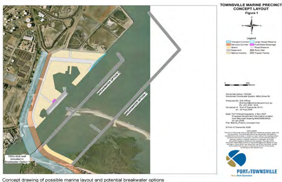
Concept drawing of possible marina layout and potential breakwater options
