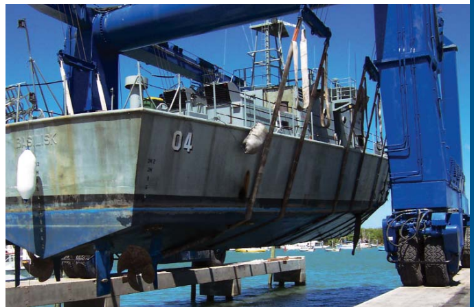
A Defence Force Pacific Patrol boat HMPNGS Basilisk is lifted for re-fit using Rosshaven Marine's recently-acquired 180 tonne ship lift.
