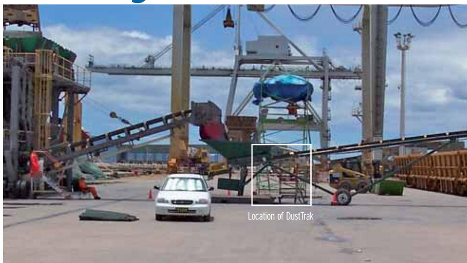
Figure 2. Location of the DustTrak for air quality monitoring on Berth 3 during zinc concentrate unloading.
