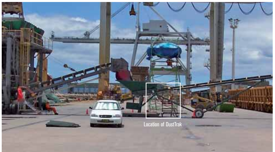
Figure 2. Location of the DustTrak for air quality monitoring on Berth 3 during zinc concentrate unloading.
