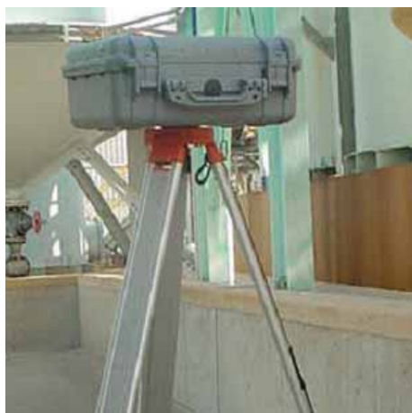
Figure 1. DustTrak™ Environmental Enclosure set-up
